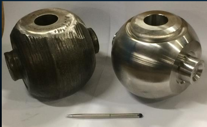
Stellite cladded valves
